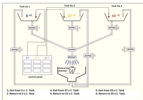
**Figure 1.** Designing the initial plan of the DSU
