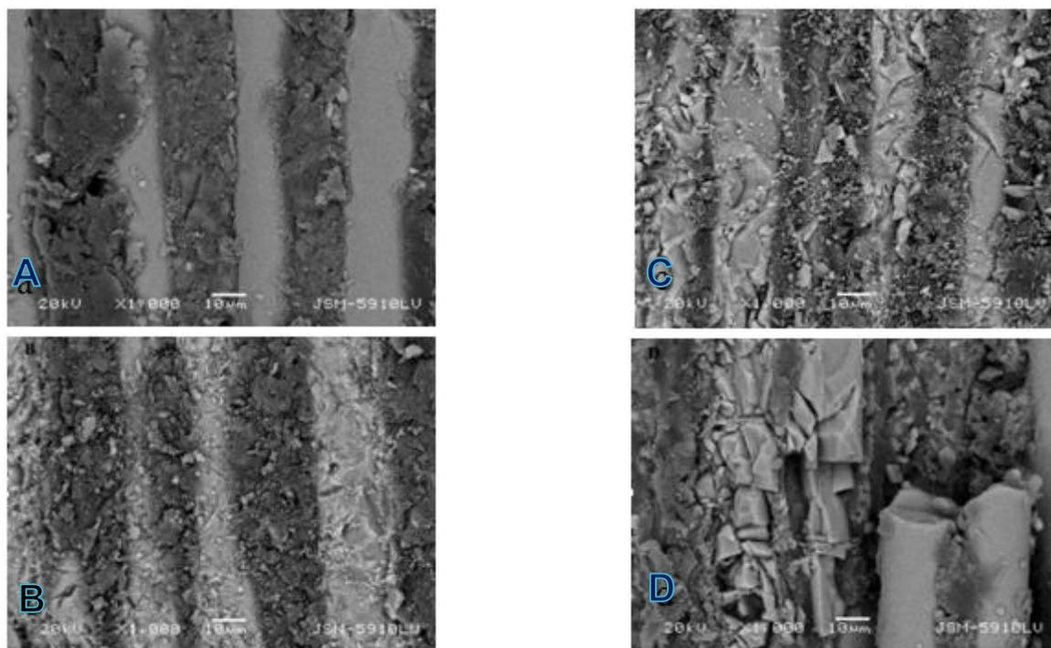
**Figure 1.** SEM images of post surfaces after surface treatment at X1000 magnification A= Control group, B= CoJet Sandblasting, C= Al<sub>2</sub>O<sub>3</sub> Sandblasting, and D=YbPL Laser
