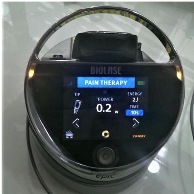
Figure 1. The employed diode laser (Epic 10, Biolase, Irvine, CA, USA) at a calibrated power of 0.2 W, emitting a pulsed light at a wavelength of 940 nm, energy of 2J and energy density of 2.5 J/cm<sup>2</sup>.
