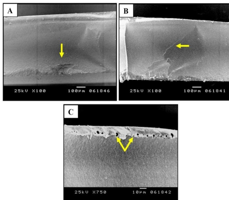
**Figure 4.** A: Scanning electron microscope (SEM) of fractured surface of zirconia-reinforced lithium silicate (ZLS) glazed specimens, crack origins mainly semi-elliptical flaws on surface at  $\times 100$ ; B: SEM of fractured surface of ZLS glazed specimens; arrows indicating crack direction propagation at  $\times 100$ ; C: SEM of glazed Celtra Duo samples with some micropores (arrows) present at interface between glaze layer and upper surface of disc at  $\times 750$
