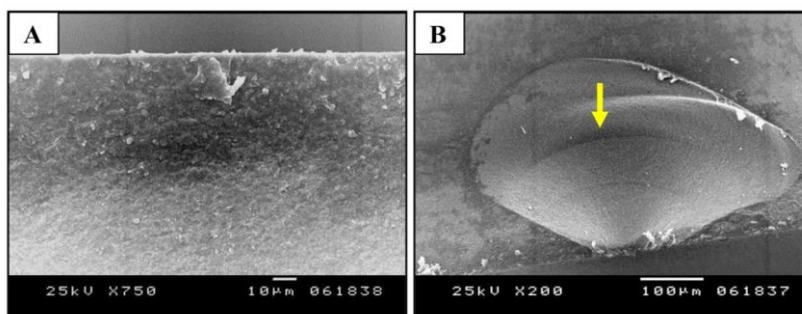
**Figure 5.** A: Scanning electron microscope of fully-crystallized polished Celtra Duo (zirconia-reinforced lithium silicate) material showing fine grain structure of material at  $\times 750$  magnification; B: another photomicrograph of zirconia-reinforced lithium silicate Celtra Duo polished specimens with visible hackle lines (arrow) at site of crack origin at  $\times 100$
