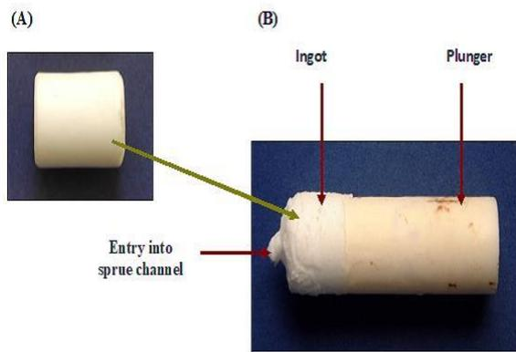
**Figure. 6A-B.** (A) - HG0.5 glass-ceramic ingot before pressing. (B) -The pressed glass ingot, subsequently cerammed, showing a small amount of pressed material with the plunger still attached
