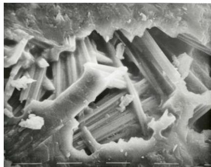
**Figure 4.** SEM of a fracture surface showing some needle-like crystals
