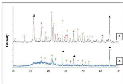
**Figure 3.** XRD of HG0.5 that were subjected to heat treatment (A) to form fluorapatite and (B) to form Apatite-mullite (▲ Aluminium, ♦ Fluorapatite, \* Mullite and Δ Cristobalite)
