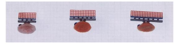
Figure 1. Three-, five-, and six-unit wax specimens with a dot on crucible former
