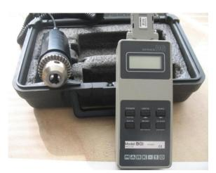
Figure 2. The Mark-10 electronic torque measurement device
