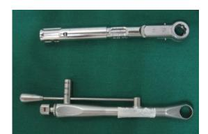
**Figure 1.** Examples of a friction wrench (above) and a spring wrench (below)
