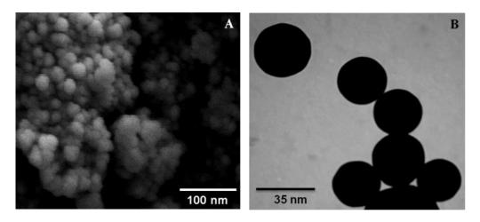
Figure 1. (A) SEM photography of TiO2 nanoparticles, (B) TEM photography of TiO2 nanoparticles
