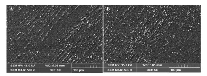
Figure 3. SEM images taken from cross-section of (A) Beautifil Flow with 0.5% TiO<sub>2</sub> nanoparticles and (B) Clearfil AP-X Flow with 0.5% TiO<sub>2</sub> nanoparticles 0.5 wt%
