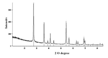
Figure 2. XRD report of TiO<sub>2</sub> nanoparticles
