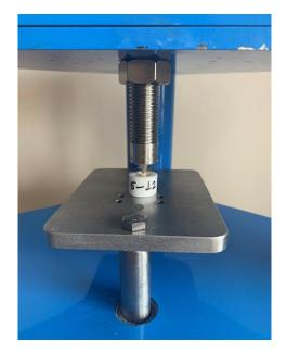
Figure 1. Fracture strength test apparatus.
