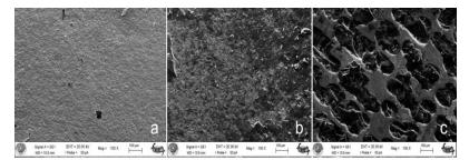
**Figure 2.** SEM Micrographs of Zirconia Surface: a) Group C, b) Group SB, c) Group B
