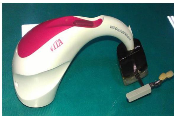
**Figure 2.** Spectrophotometer in acrylic holder
