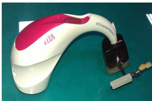
**Figure 2.** Spectrophotometer in acrylic holder
