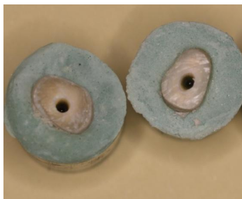
Figure 1. Two prepared samples before post cementation
