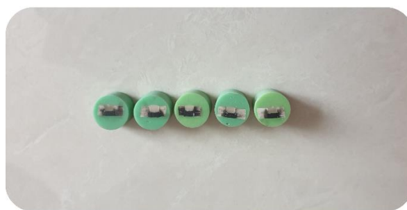
Figure 2. Samples prepared for Vickers microhardness testing
