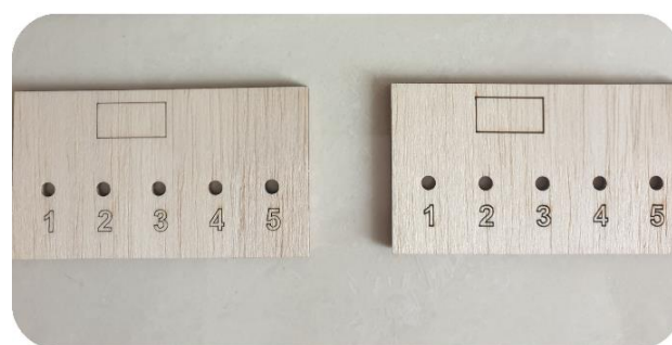
Figure 1. Custom wooden molds for sample preparation
