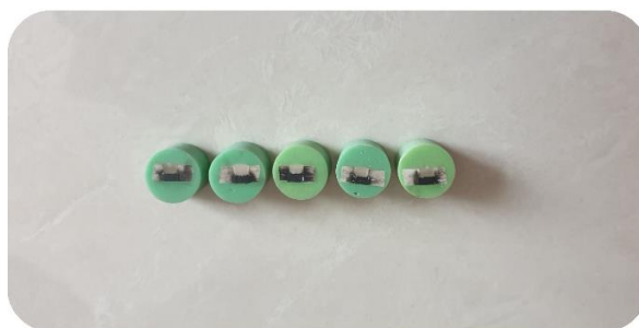
Figure 2. Samples prepared for Vickers microhardness testing
