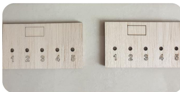
Figure 1. Custom wooden molds for sample preparation
