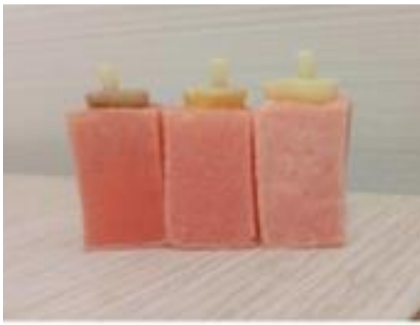
Figure 1. Mounted dental specimens in acrylic resin
