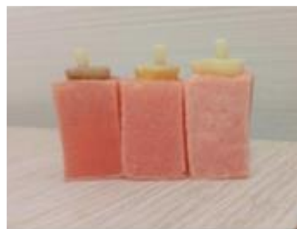
Figure 1. Mounted dental specimens in acrylic resin
