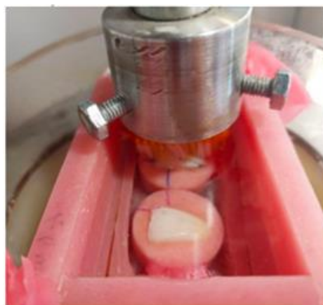
Figure2. The artificial mouth device and the toothbrushing simulator used in this study
