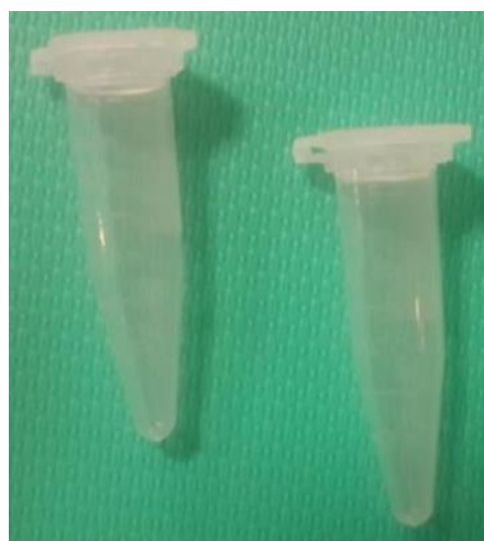
Figure 2. Microtubes used for direct contact testing (DCT) to assess the antimicrobial properties of sealers
