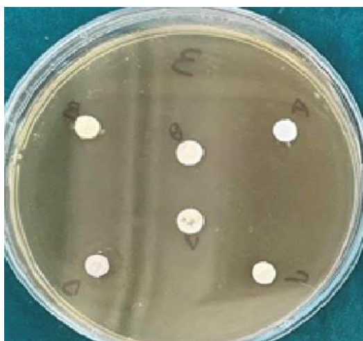
Figure 1. Agar diffusion test (ADT) performed on a Brain Heart Infusion (BHI) agar plate with wells containing sealer discs
