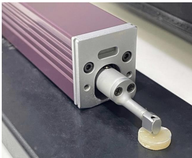
Figure 3. Evaluating the surface roughness value of the composite disk specimen using the SJ-310 Mitutoyo stylus profilometer
