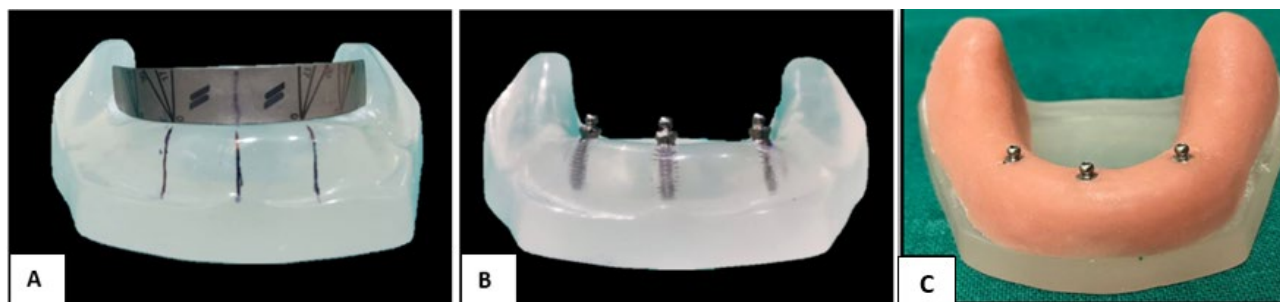
Figure 1. (A) Angulation assessment of implant sites using a planning guide; (B) Three parallel implants placed in the mandibular model; (C) Auto-polymerized silicone resilient liner simulating mucosa, with ball abutments (male parts) exposed
