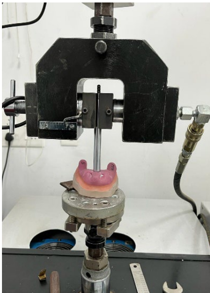
Figure 4. The universal testing machine (UTM) setup for evaluating the retentive force of attachment systems
