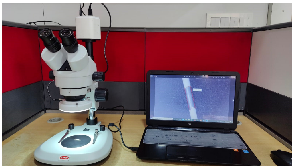
Figure 2. The stereomicroscope and Capture 2.3 software used for coating loss measurement
