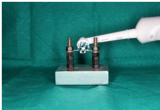
Figure 1. The experimental stand securing the wire and applying mechanical stress using an electric toothbrush
