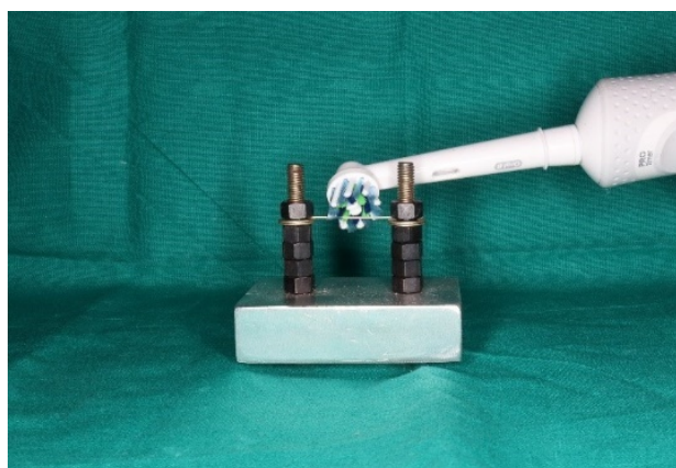
Figure 1. The experimental stand securing the wire and applying mechanical stress using an electric toothbrush
