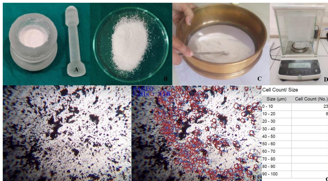
Figure 1. Egg shell powder preparation and particle size analysis. A) Mortar and pestle; B) Egg shell powder; C) Egg shell powder passed through a sieve; D) measuring the weight of egg shell powder; E) A microscopic image showing the unprocessed microstructure of egg shell powder, highlighting the particle size and distribution; F) A microscopic image with cell count analysis, red circles indicating the particle size; G) The Cell Count/Size table summarizing the cell count based on the size of powder particles in micrometers (µm) and demonstrating the distribution of different cell sizes.
