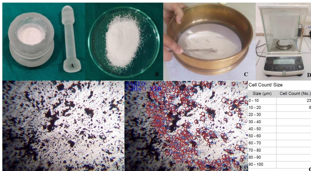
Figure 1. Egg shell powder preparation and particle size analysis. A) Mortar and pestle; B) Egg shell powder; C) Egg shell powder passed through a sieve; D) measuring the weight of egg shell powder; E) A microscopic image showing the unprocessed microstructure of egg shell powder, highlighting the particle size and distribution; F) A microscopic image with cell count analysis, red circles indicating the particle size; G) The Cell Count/Size table summarizing the cell count based on the size of powder particles in micrometers ( \mu\text{m} ) and demonstrating the distribution of different cell sizes.
