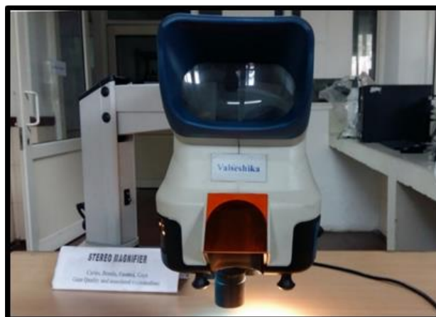
Figure 2. The stereomicroscope used for scoring Adhesive Remnant Index (ARI)
