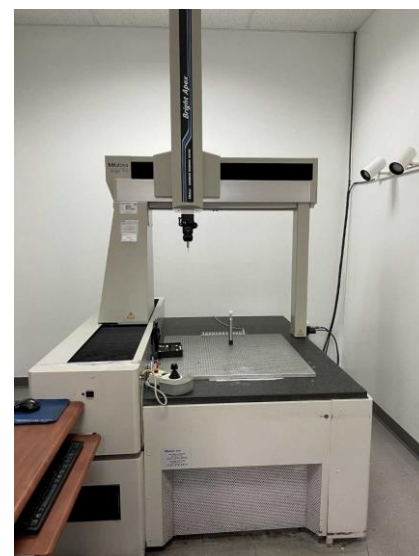
Figure 6: The coordinate measuring machine with its probe and two horizontal and vertical arms
