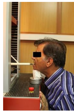
Figure 4: Fixing the patient's head in front of the retention measurement device, using a chin holder adjusted based on the patient's height
