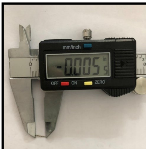
Figure 2: Measurement of the fractured fragment using a digital Vernier caliper
