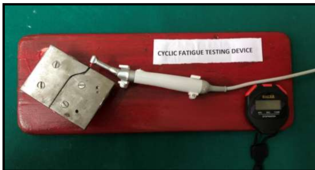
Figure 1: The cyclic fatigue testing device with a supported handpiece
