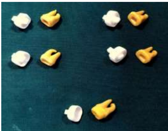
Figure 2. Printed resin specimens and zirconia copings for each group
