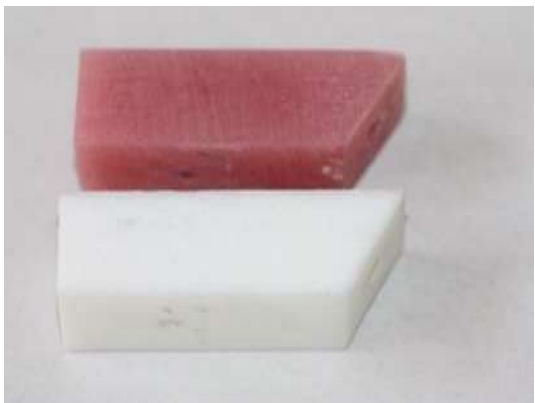
Figure 4. The designed jig for angular tensile force
