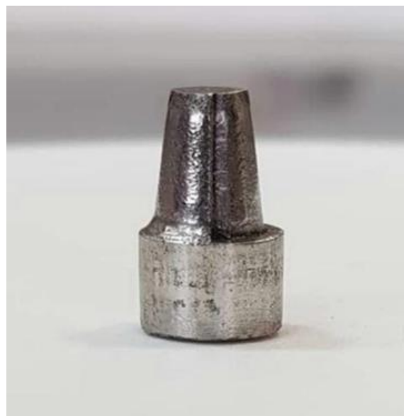
Figure 1: The chrome-cobalt standard die with two cervical finish lines
