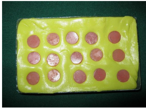
Figure 4. 10-mm heat cure disc pressed on silicone material
