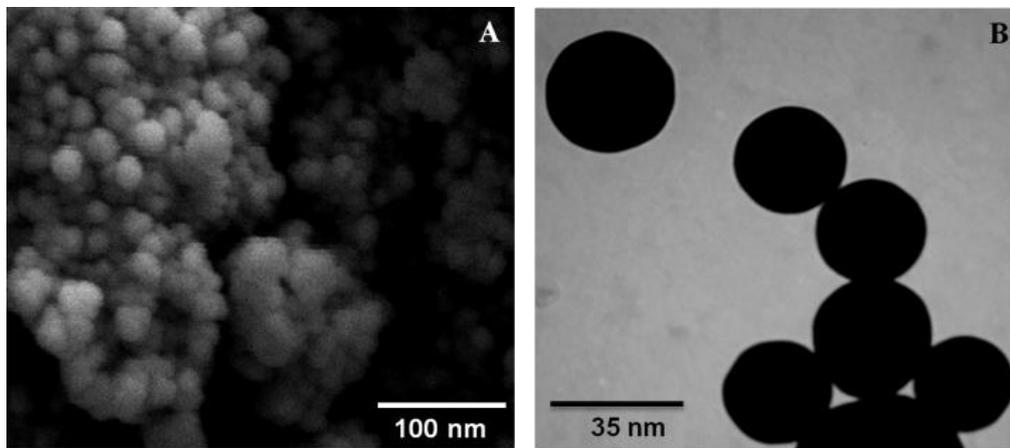
**Figure 1.** (A) SEM photography of TiO<sub>2</sub> nanoparticles, (B) TEM photography of TiO<sub>2</sub> nanoparticles
