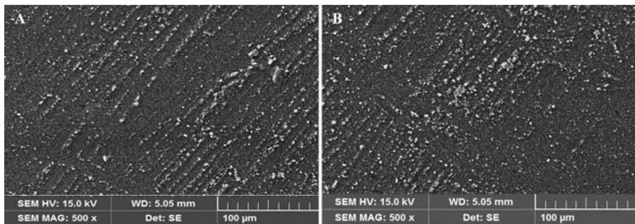
**Figure 3.** SEM images taken from cross-section of (A) Beautifil Flow with 0.5% TiO<sub>2</sub> nanoparticles and (B) Clearfil AP-X Flow with 0.5% TiO<sub>2</sub> nanoparticles 0.5 wt%
