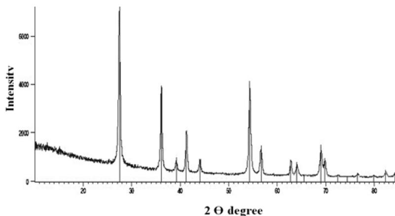
**Figure 2.** XRD report of TiO<sub>2</sub> nanoparticles
