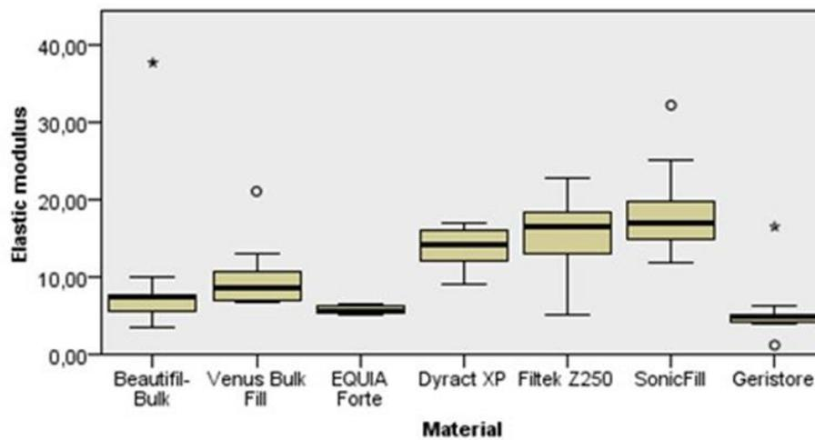
**Figure 3.** Box plot graphic of Er scores of all tested materials.
