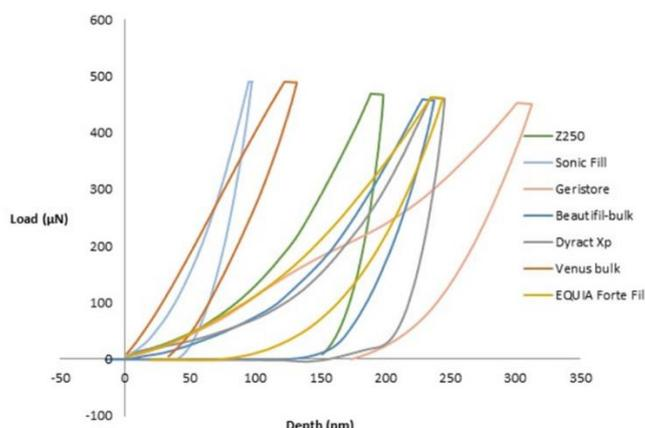
Figure 1. Load-depth curves of the one sample from each group of tested materials.
