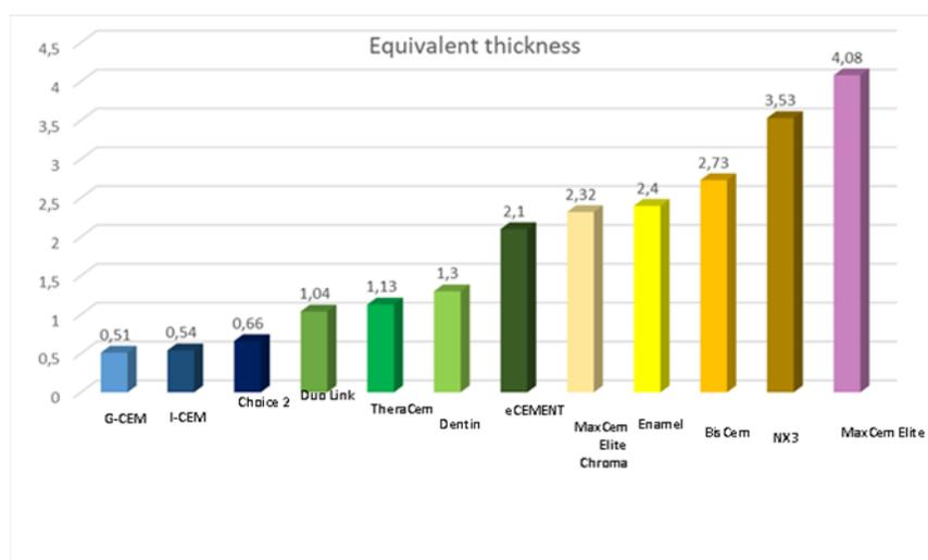
Figure 3: The equivalent aluminum thickness value of each sample
