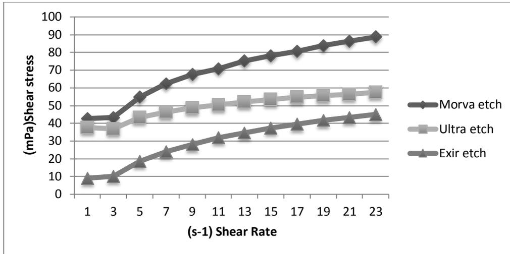
Figure 1: Shear stresses of the evaluated acids at different shear rates.
