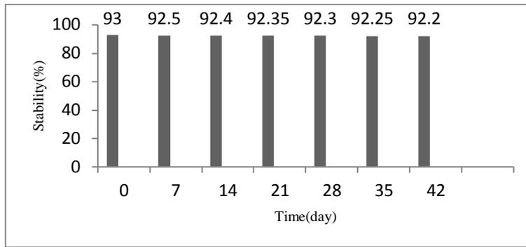
Figure 3. Stability of the Exir acid etchant.
