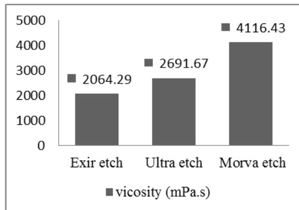
Figure 2: Viscosity of the evaluated acid etchants at a shear rate of 21 per second.
