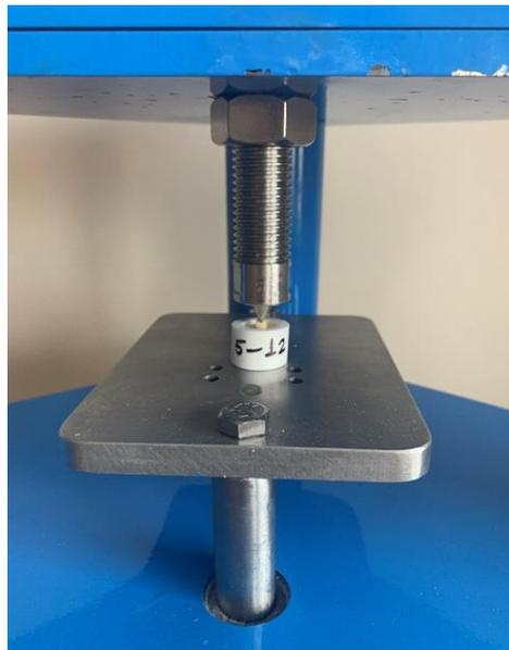
Figure 1. Fracture strength test apparatus.
