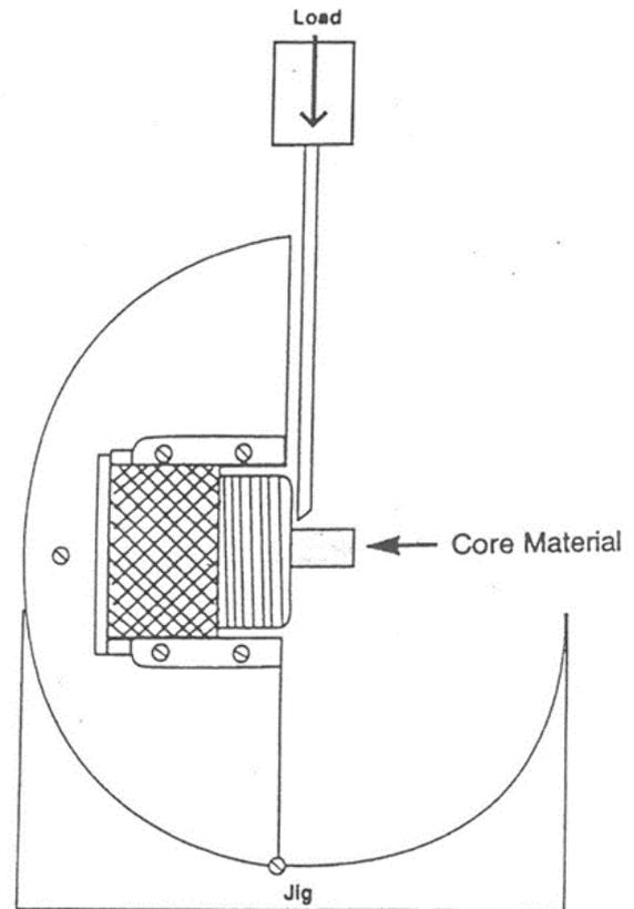
Figure 4. Schematic image of the sample in the fixture specific for the tester device and the angle of exerted force
