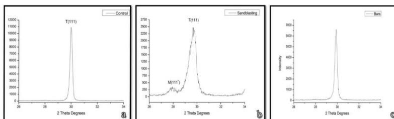
**Figure 4.** XRD Analysis of Zirconia: a) Group C, b) Group SB, c) Group B
