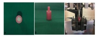
Figure 1: A single specimen tested in the study C: Specimens subjected to bond strength testing in a universal testing machine
