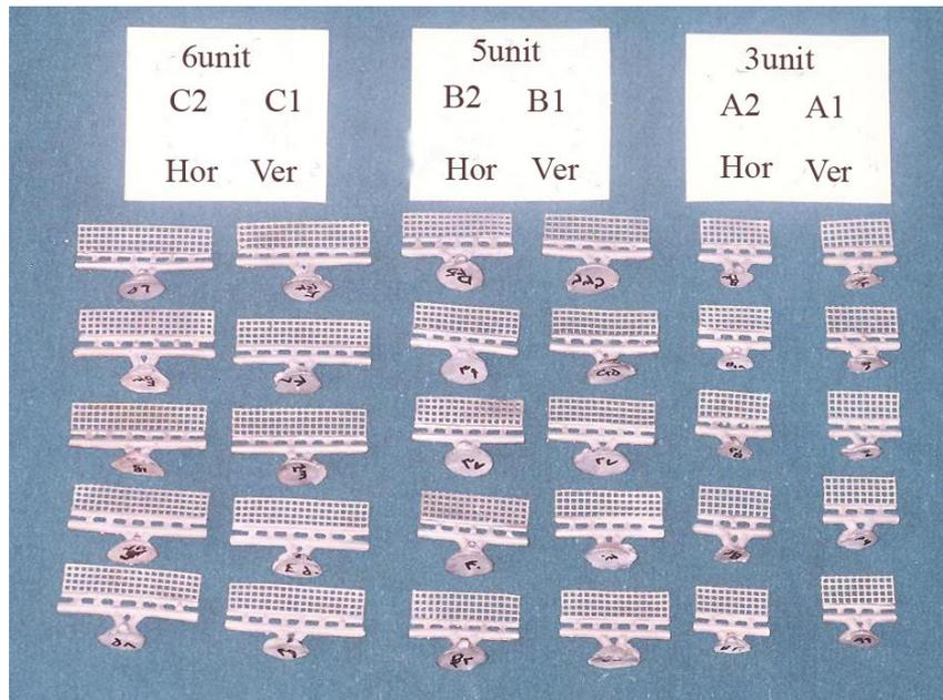
**Figure 2.** Casted bridge specimens in vertical and horizontal situation after sandblasting
