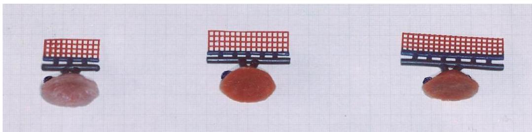
**Figure 1.** Three-, five-, and six-unit wax specimens with a dot on crucible former
