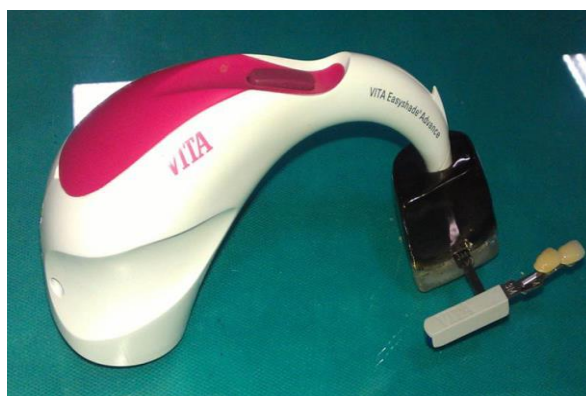
Figure 2. Spectrophotometer in acrylic holder
