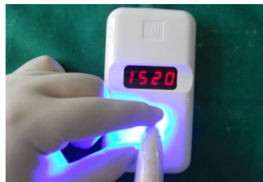
Figure 2. LED radiometer used to record the intensity output
