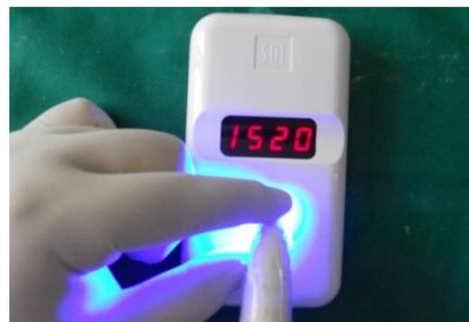
Figure 2. LED radiometer used to record the intensity output
