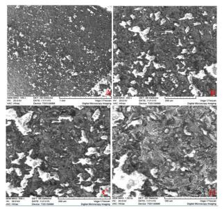
Figure 2. SEM images of the fractured surfaces of sandblasted specimens (×100, ×300, ×500 and ×1000 magnifications).
