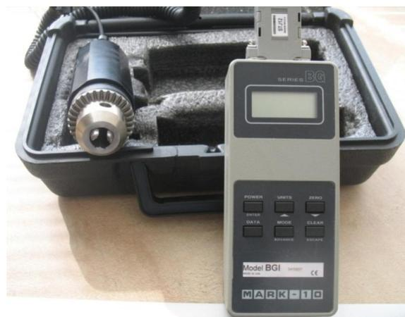
**Figure 2.** The Mark-10 electronic torque measurement device
