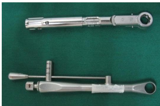
**Figure 1.** Examples of a friction wrench (above) and a spring wrench (below)
